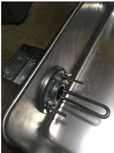
Photos 9-11: Germination Chamber - heat provided by hot water heater element wired into waterproof thermostat inside chamber - chamber can germinate 4080 plants at one time!
