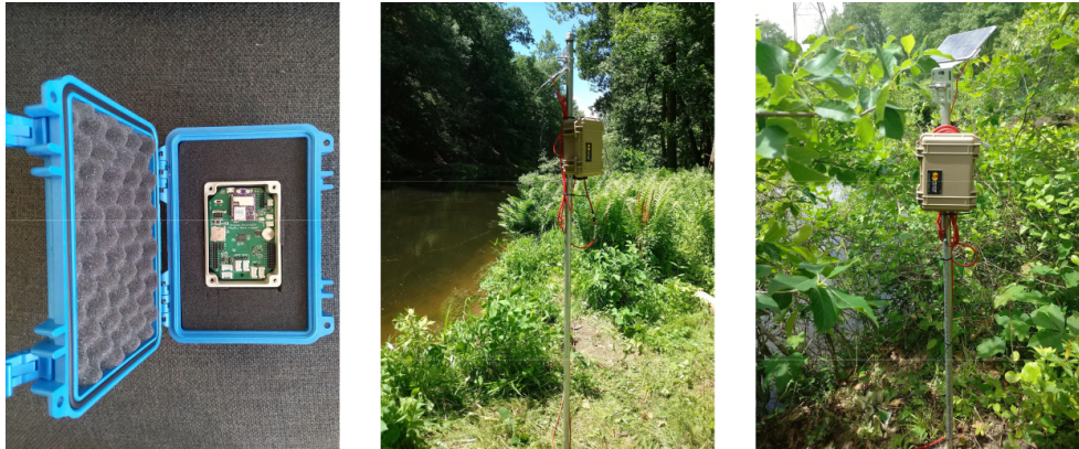
Close-up image of the inside of a water monitoring station; and stations 1 and 2, located on the Lower Basha Kill. The stations are checked monthly by our trained volunteers, and are reliable year-round in ordinary weather conditions.
